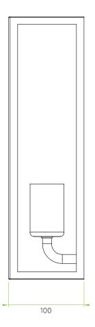
Recess in wall for Terminal Block 60x60x30mm
